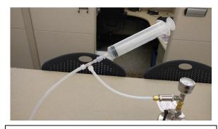
Photograph 14: Use of syringe to purge air from tubing and below ground
