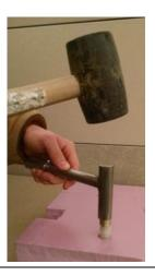
Photograph 6: Installation Tool w/ Mallet
