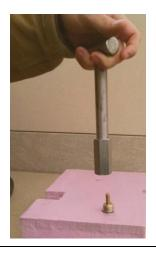
Photograph 15: Vapor Pin® Extraction
