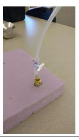
Photograph 8: Shut-In Test assembly connection to Vapor Pin®
