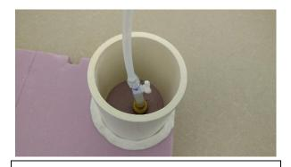
Photograph 13: Two-way valve opened to soil
