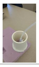
Photograph 9: Water dam around Vapor Pin®
