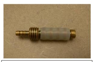
Photograph 2: Silicone tubing properly inserted onto Vapor Pin®
