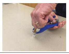
Photograph 1: Using Elastrator to push Vapor Pin® into silicone tubing
