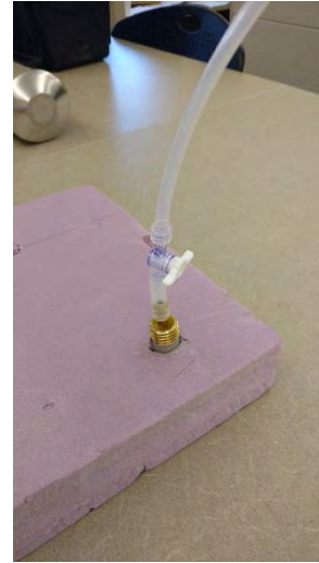
Photograph 8: Shut-In Test assembly connection to Vapor Pin®
