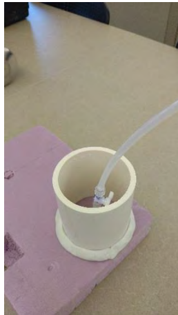
Photograph 9: Water dam around Vapor Pin®
