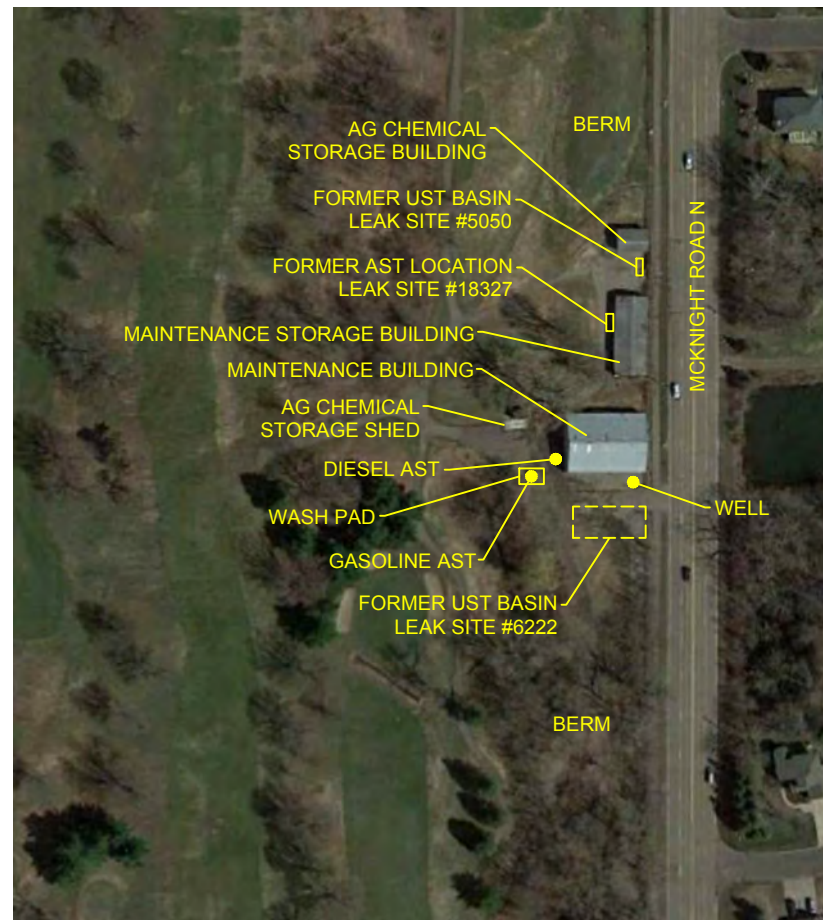
INSET 2: MAINTENANCE FACILITY SCALE: 1" = 200'
