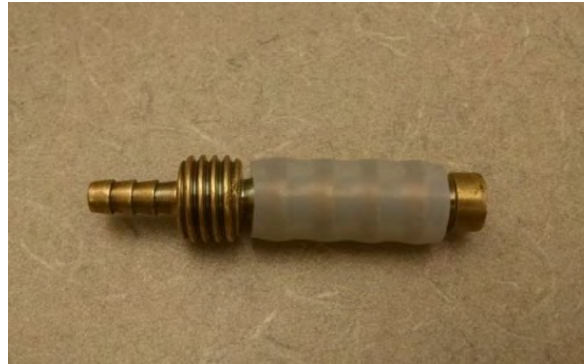
Photograph 2: Silicone tubing properly inserted onto Vapor Pin®
