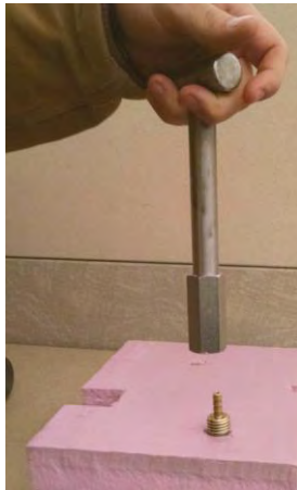
Photograph 15: Vapor Pin® Extraction
