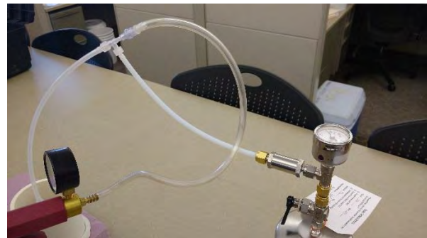
Photograph 12: Vacuum pump connected to check valve on Shut-in Test assembly
