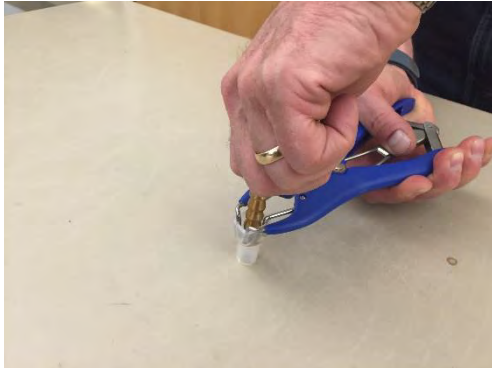
Photograph 1: Using Elastrator to push Vapor Pin® into silicone tubing
