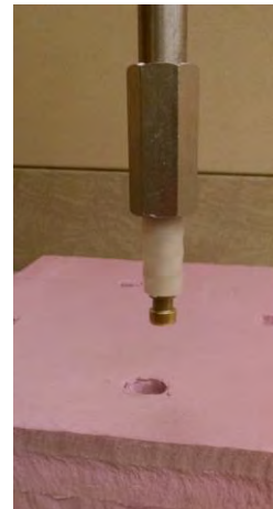
Photograph 16: Vapor Pin® Extraction
