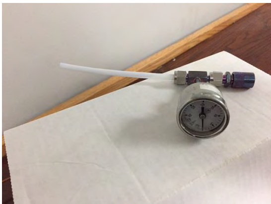
Photograph 17: Alternate gauge and valve connection assembly (courtesy Legend Laboratory)
