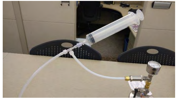
Photograph 14: Use of syringe to purge air from tubing and below ground
